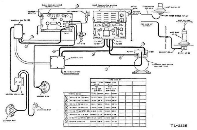
FIGURE 12.-Radio sets SCR-193-A and SCR-193-C, cording diagram.
