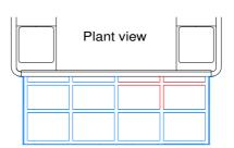
Cut the parts in red to mount the rack along the spare wheel
